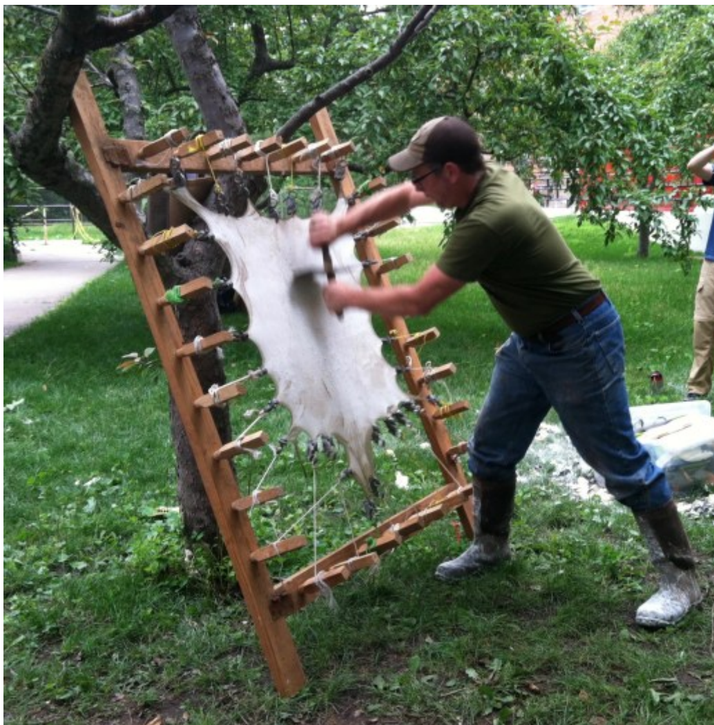
Parchment master, Jesse Meyer of Pergamena demonstrating his technique using a tool he created himself, designed after the fashion of medieval instruments. Image by author.
