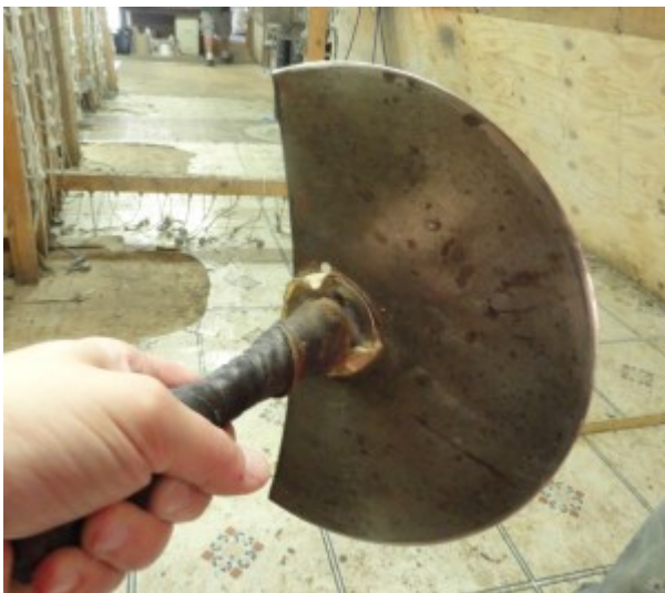
A close up of the scraping tool crafted by Jesse Meyer of Pergamena.
